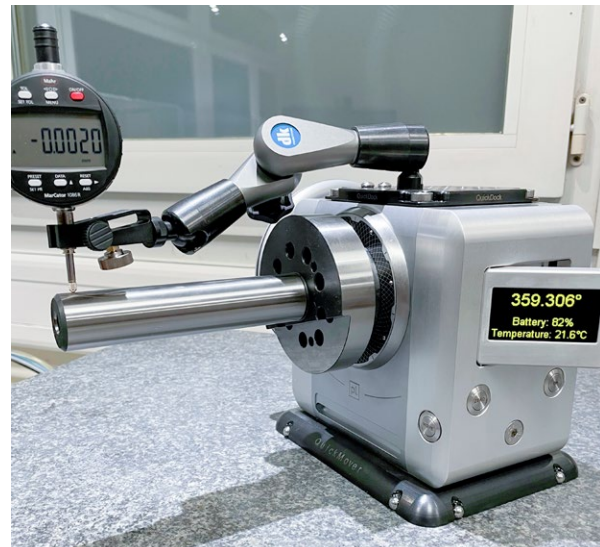
Roundness measurement with a dial gauge mounted on a grid plate. Optional dk grid plate as an ideal platform for additional tools.
